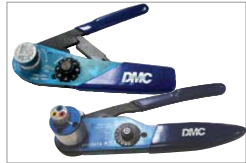
Examples of M22520 Series Crimping Tools:
