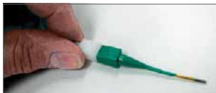
Plastic tool with contact in proper position.
