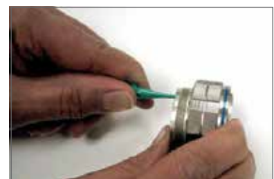
Plastic tool with contact in proper position.
