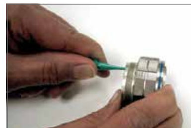
Plastic tool with contact in proper position.
