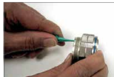
Plastic tool with contact in proper position.
