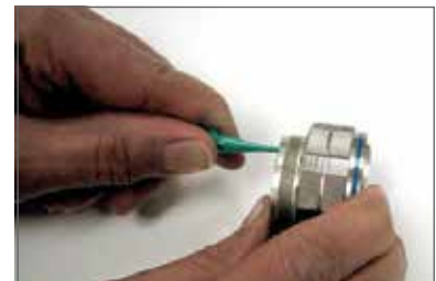
Plastic tool with contact in proper position.
