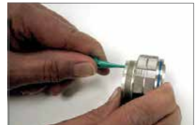
Plastic tool with contact in proper position.
