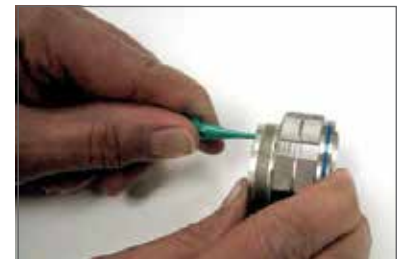
Plastic tool with contact in proper position.
