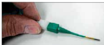
Plastic tool with contact in proper position.
