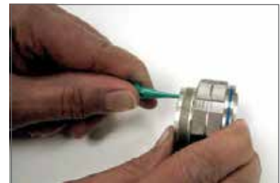
Plastic tool with contact in proper position.
