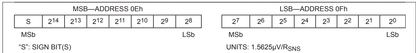
Figure 6. Current Register Format
