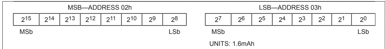
Figure 16. Remaining Active Absolute Capacity (RAAC) [mAh]
