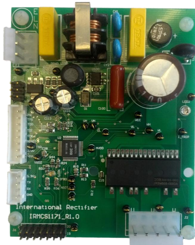
Figure 4: Reference design board featuring the \mu IPM™-DIP module and the iMotion™ IRLMCF171 digital control IC
