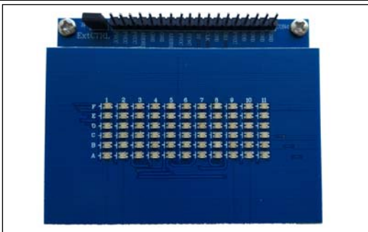
Figure 1: Photo of IS31FL3743A Evaluation Board
