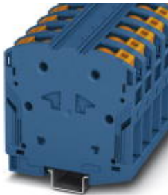
High-current terminal block, Connection method: Push-in connection, Cross section: 25 mm 2 - 95 mm 2 , AWG: 4 - 3/0, Width: 25 mm, Color: blue, Mounting type: NS 35/15
