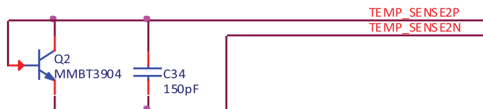
Figure 8.5. NPN Temperature Sensor Circuit
