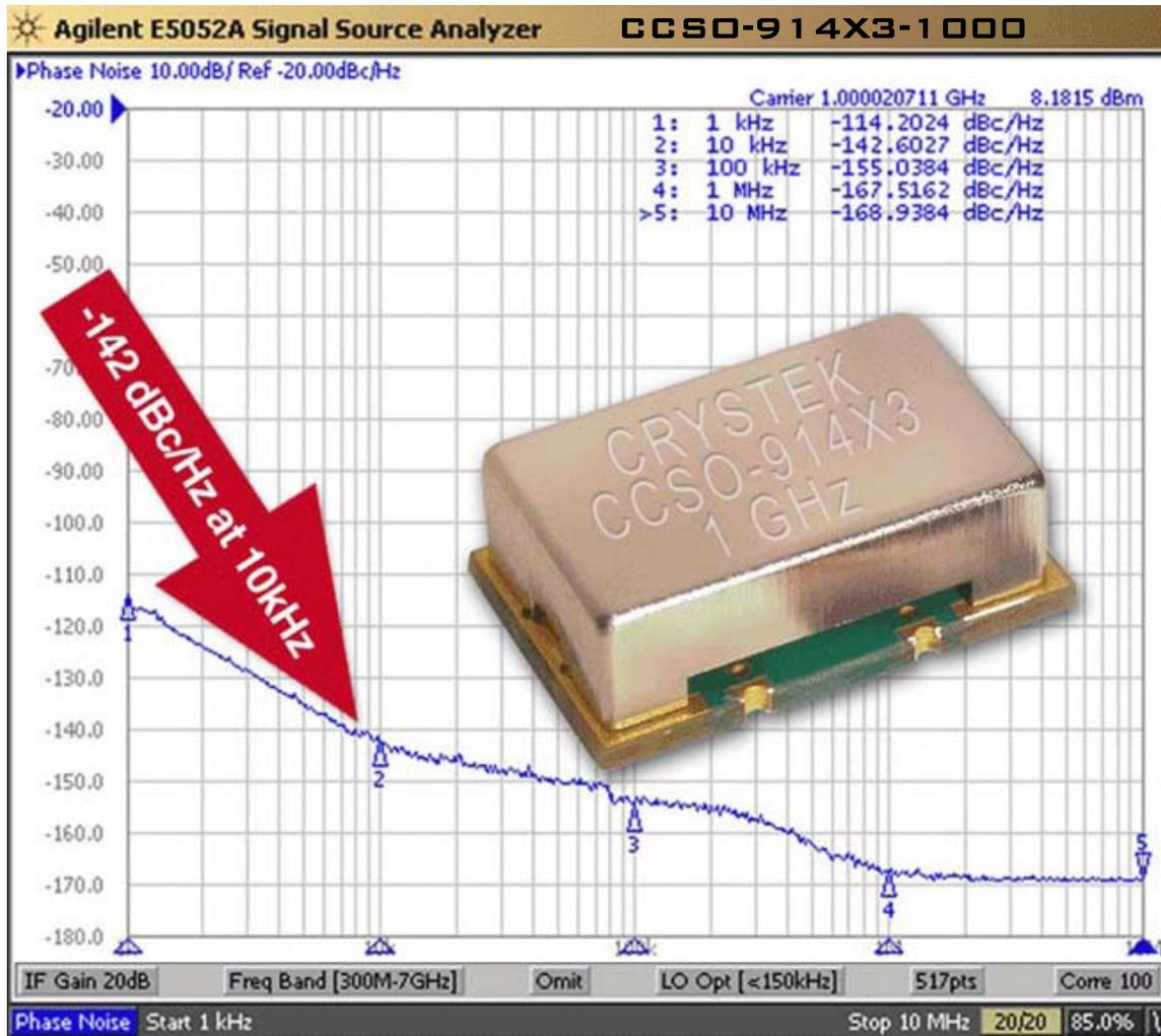
Model CCSO-914X3-1000 is a 1 GHz SAW (surface acoustic wave) Clock Oscillator (CCSO). SAW crystal technology provides low-noise and low-jitter performance with true sinewave output. Features include -142dBc/Hz phase noise at 10kHz offset, 3.3V input voltage, -40°C to +85°C operating temperature, FR5 PCB and 9×14 mm SMT package. The oscillator has no sub-harmonic and the second harmonic is typically -25dBc.
