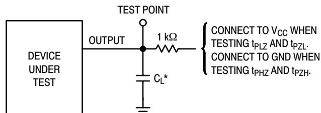
\*Includes all probe and jig capacitance
