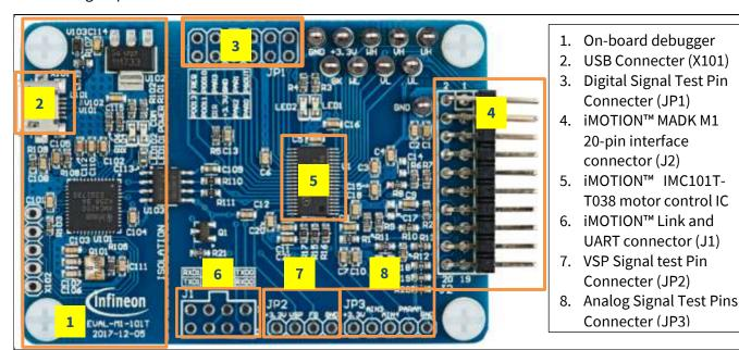
Figure 4 Functional groups of the EVAL-M1-101T evaluation board's top side
