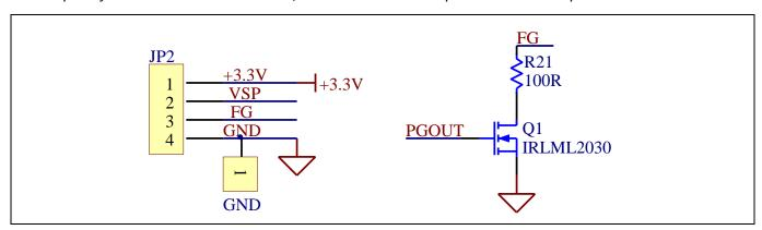
Figure 23 VSP Input Connector and level shit schematic for FG
