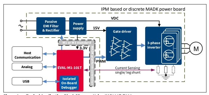
Figure 2 Typical Application Block Diagram Using IMC101T-T038
