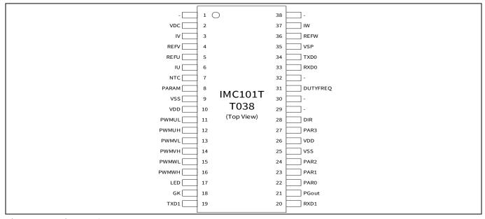
Figure 3 Pinout of IMC101T-T038
