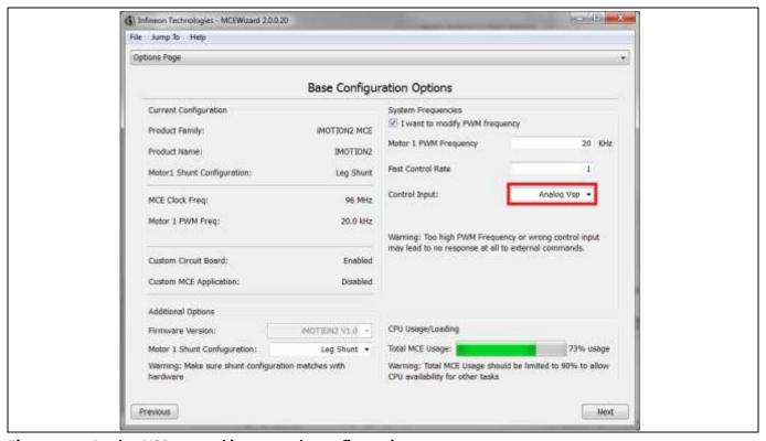
Figure 19 **Analog VSP control input mode configuration**
