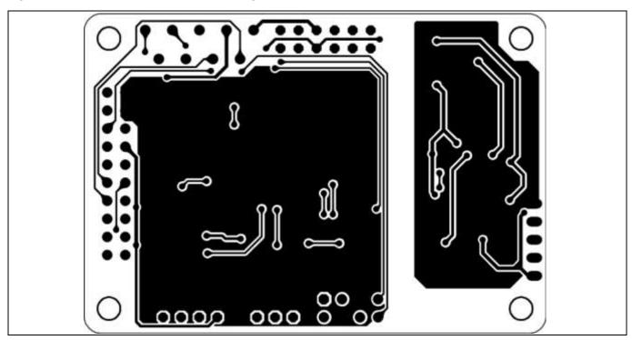
Figure 29 Bottom layer routing of the EVAL-M1-101T
