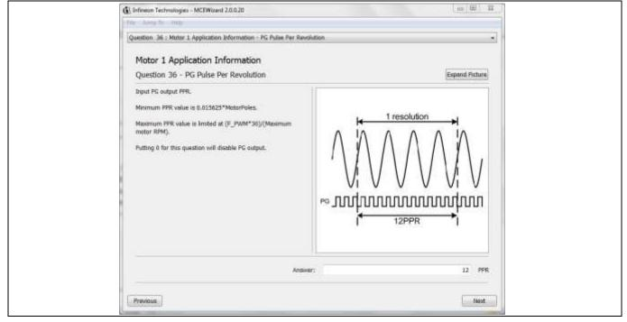
Figure 22 PG Pulse Per Revolution configuration
