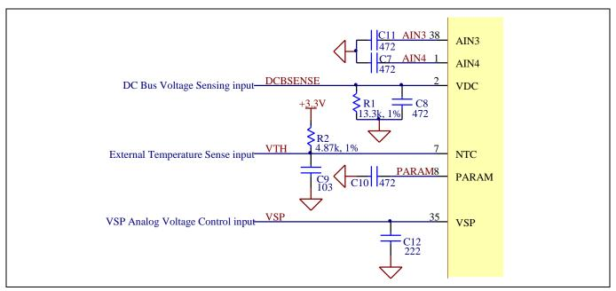
Figure 16 Analog inputs on the EVAL-M1-101T evaluation board
