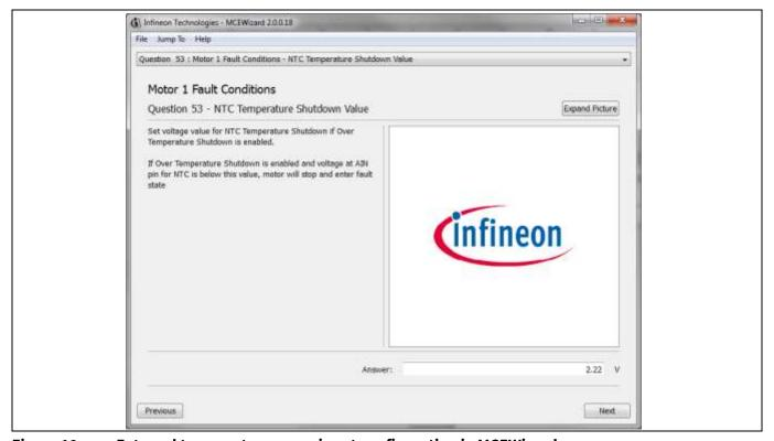
Figure 18 External temperature sense input configuration in MCEWizard
