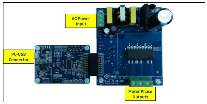
Figure 5 System connection example using EVAL-M1-101T and EVAL-M1-05-65D
