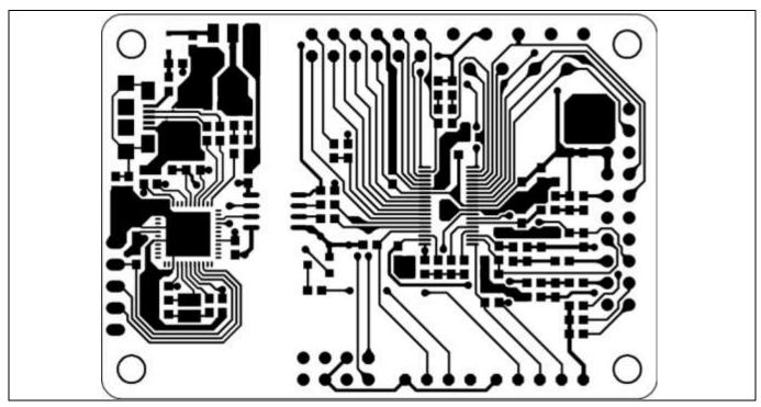
Figure 28 Top layer routing of the EVAL-M1-101T
