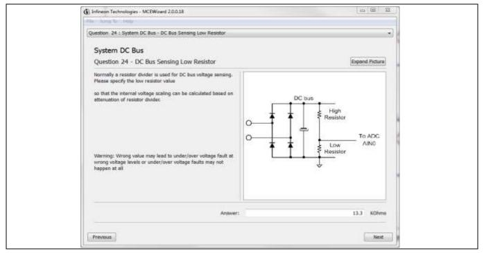
Figure 17 DC bus sensing configuration in MCEWizard
