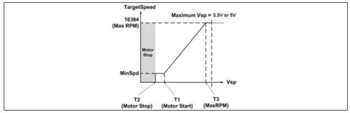
The relationship between VSP Analog Input voltage and TargetSpeed Figure 20
