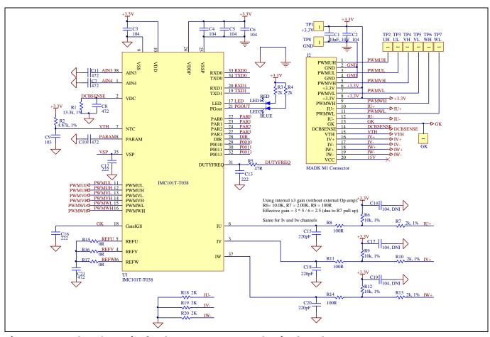
Figure 24 The schematics for the EVAL-M1-101T evaluation board
