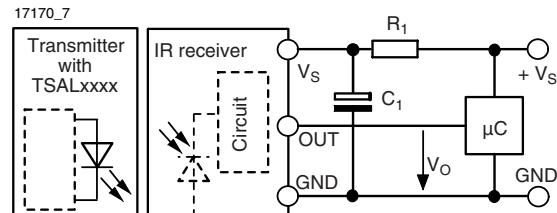
The external components  $R_1$  and  $C_1$  are optional to improve the robustness against electrical overstress (typical values are  $R_1 = 100 \Omega$ ,  $C_1 = 0.1 \mu\text{F}$ ).
