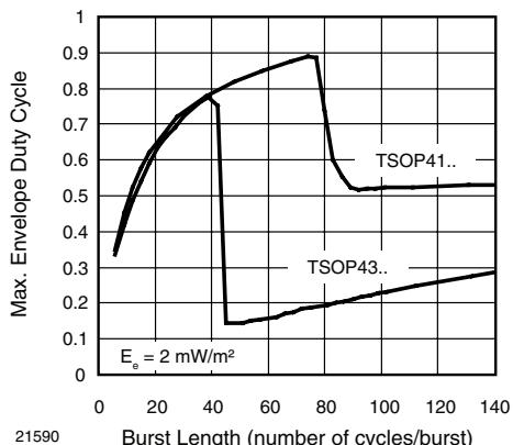
Fig. 9 - Max. Envelope Duty Cycle vs. Burst Length
