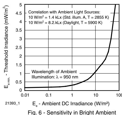
Fig. 6 - Sensitivity in Bright Ambient
