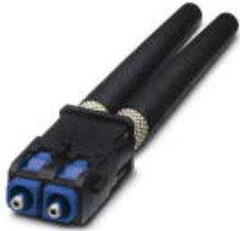
SC-RJ fiber optic connector, IP20, duplex, with fast connection technology, for polymer fiber 980/1000  $\mu\text{m}$ , for individual wire diameter 2.2 mm
