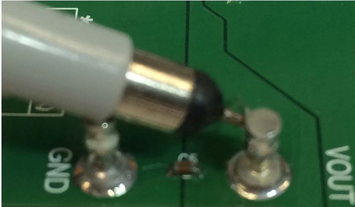
Figure 3. Output Ripple Measurement Technique
