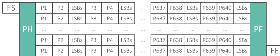
Figure 19: Example of pixel ordering for one full frame transmission
