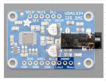
The exciting part! This is where your line level audio comes out. We put big 47uF blocking capacitors on the output so you can connect this to any stereo system. **AGND** is a clean analog ground signal that we recommend using as your analog reference, you'll get a cleaner signal.
