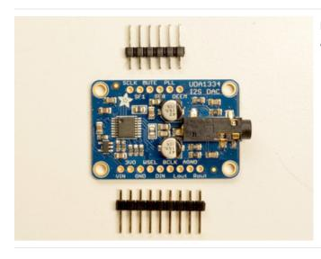
Break apart the 0.1" header into 6 and 9-pin long pieces and slip the short ends into the holes in the board
