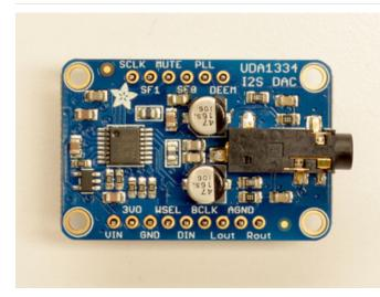
Make sure that all of the short parts of the header are sticking through the two sets of pads on either side of the board
