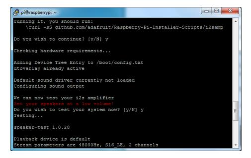
If it sounds really distorted, it could be the volume is too high. However, in order to have volume control appear in Raspbian desktop or Retropie you must reboot a second time after doing the speaker test, with **sudo reboot**
