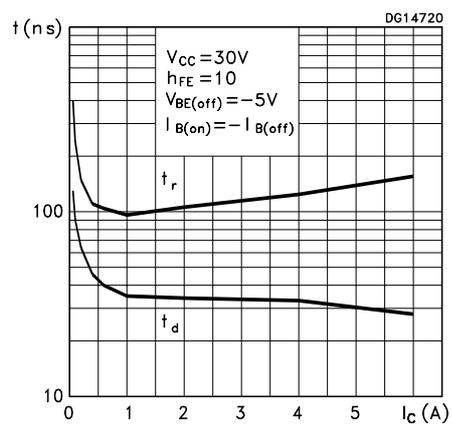
**Figure 13. Resistive Load Switching Time (NPN)**
