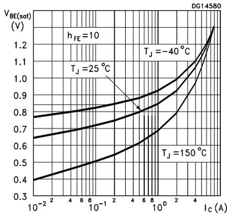
Figure 8. Base-Emitter Saturation Voltage (PNP)
