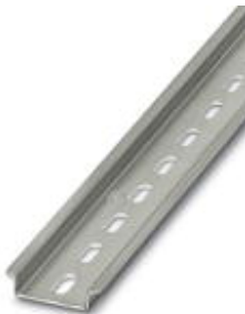
DIN rail, material: steel galvanized and passivated with a thick layer, perforated, height 7.5 mm, width 35 mm, length: 955 mm
