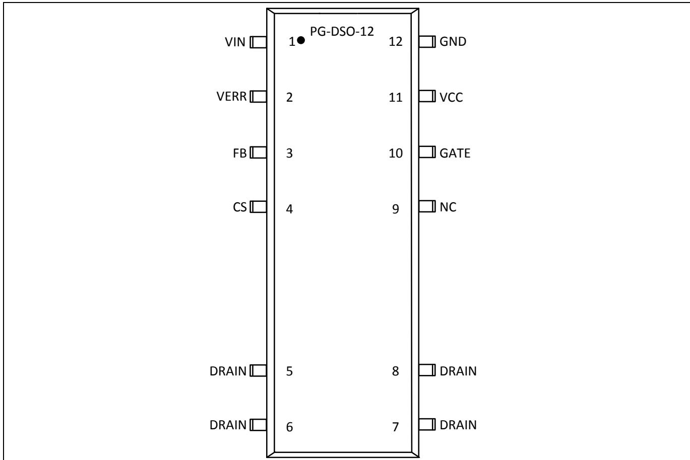
Figure 3 Pin configuration
