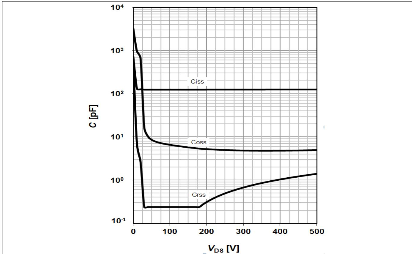
Figure 31 Typical CoolMOS™ capacitances of ICE5GR2280AG ( $C=f(V_{DS})$ ;  $V_{GS}=0$  V;  $f=250$  kHz)
