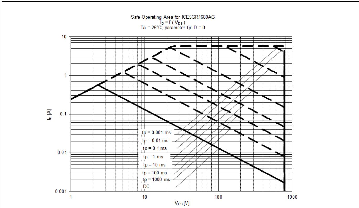
Figure 20 Safe Operating Area (SOA) curve for ICE5GR1680AG
