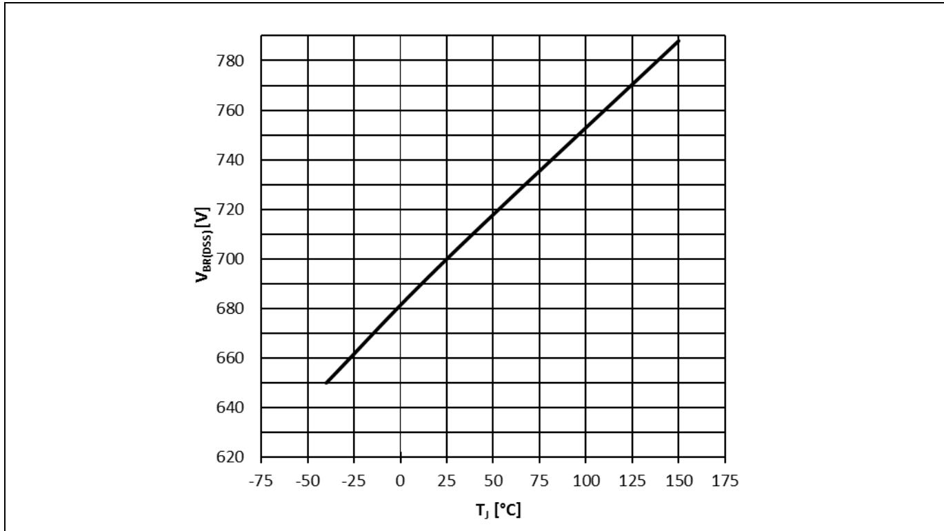
Figure 27 Drain-source breakdown voltage ICE5xRxx70AG;  $V_{BR(DSS)}=f(T_J)$ ,  $I_D=1$  mA
