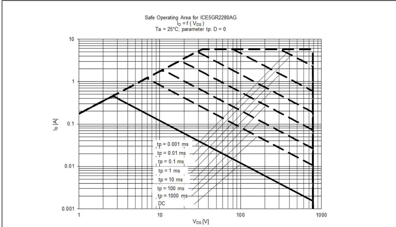
Figure 19 Safe Operating Area (SOA) curve for ICE5GR2280AG
