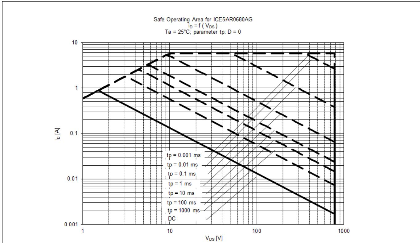
Figure 21 Safe Operating Area (SOA) curve for ICE5AR0680AG
