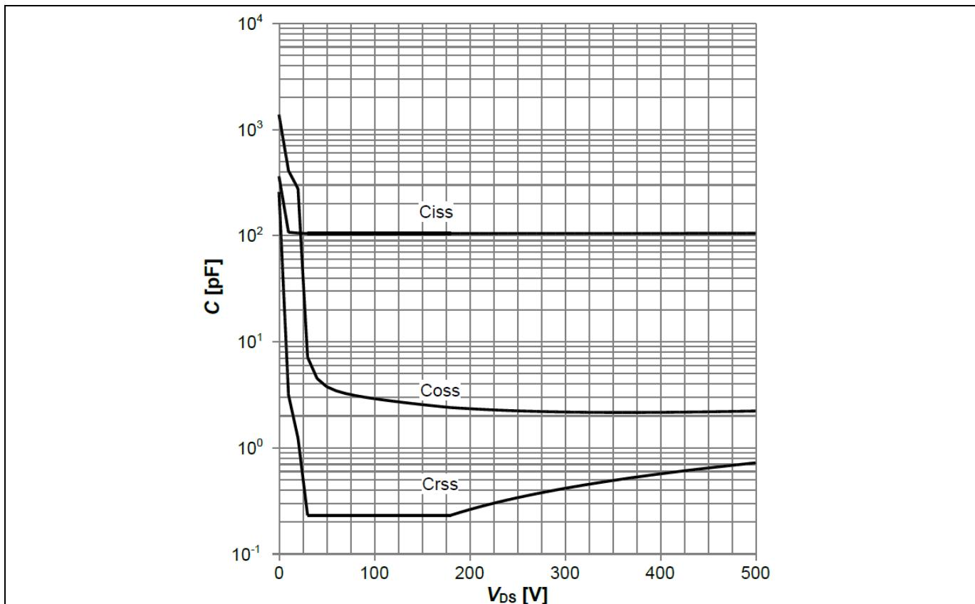
Figure 30 Typical CoolMOS™ capacitances of ICE5GR4780AG ( $C=f(V_{DS})$ ;  $V_{GS}=0$  V;  $f=250$  kHz)
