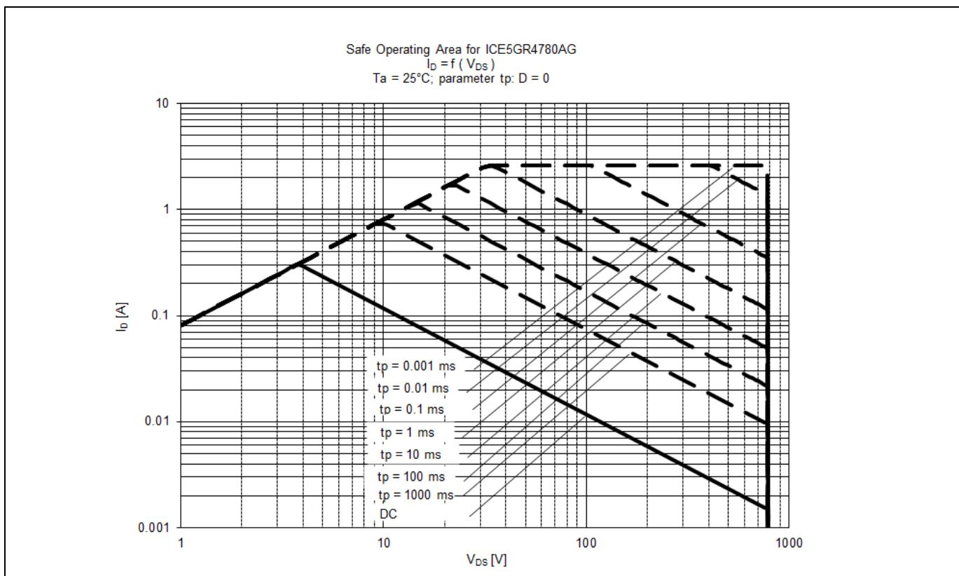
Figure 18 Safe Operating Area (SOA) curve for ICE5GR4780AG
