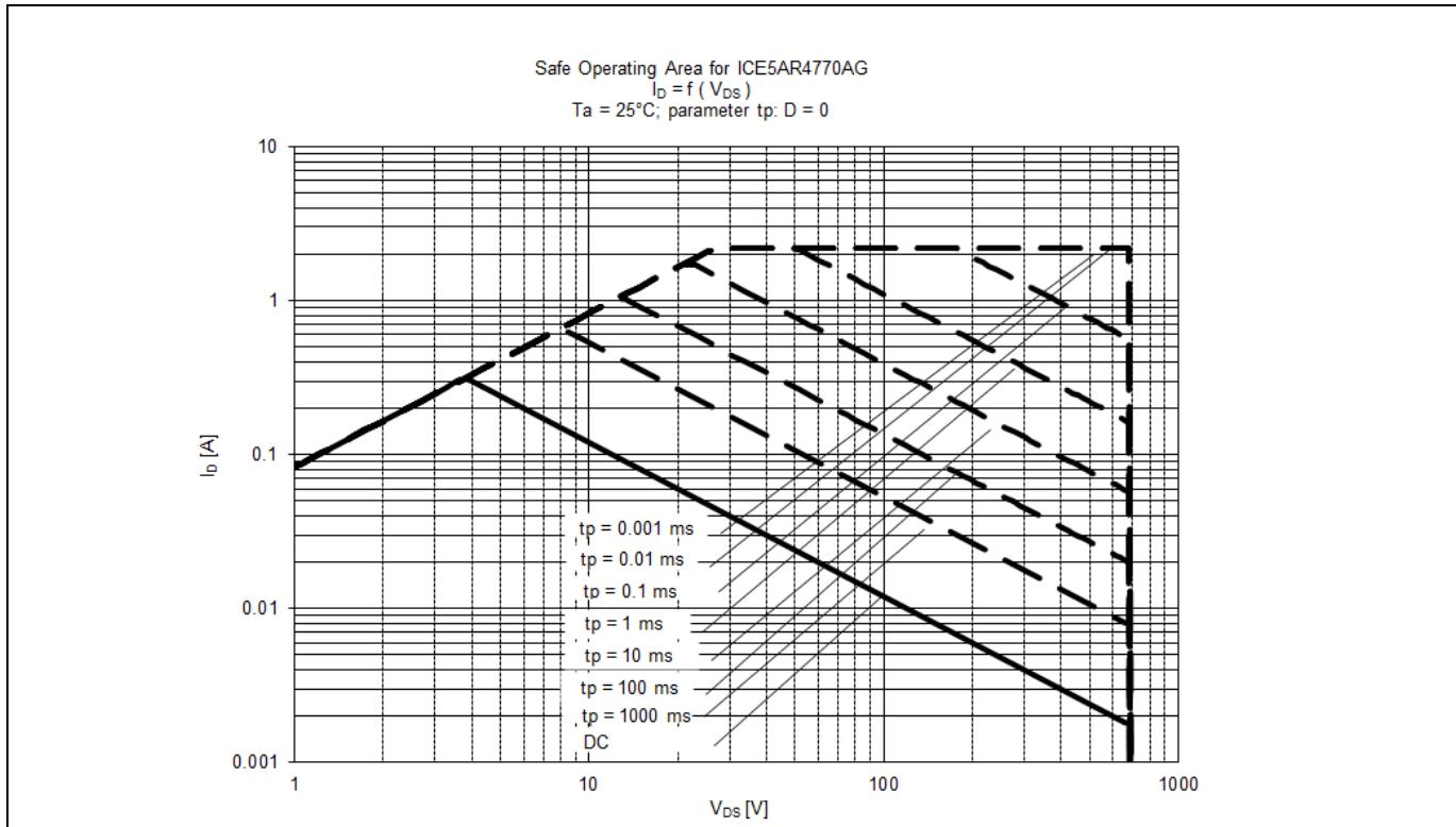
Figure 17 Safe Operating Area (SOA) curve for ICE5AR4770AG
