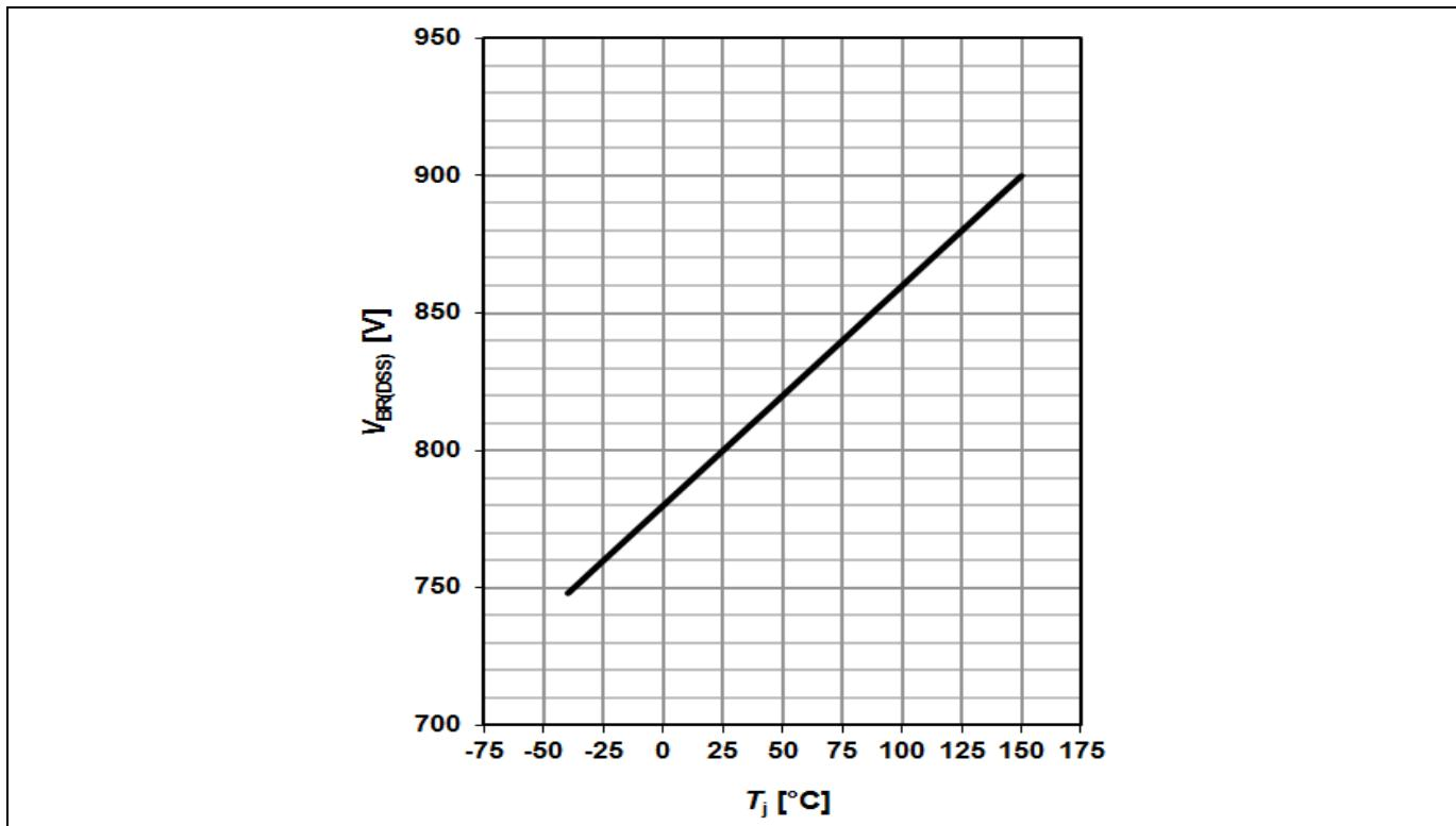
Figure 28 Drain-source breakdown voltage ICE5xRxx80AG;  $V_{BR(DSS)}=f(T_J)$ ,  $I_D=1$  mA
