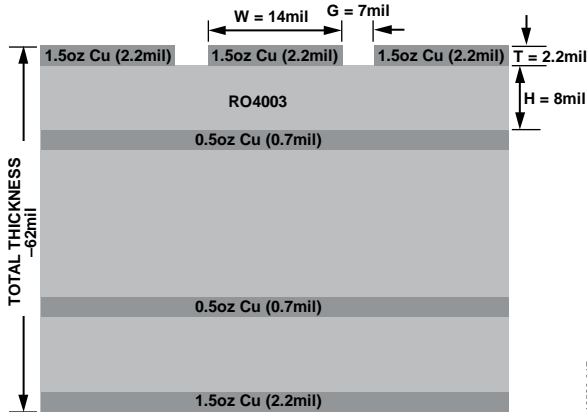
Figure 17. Evaluation Board (Cross Section View)
