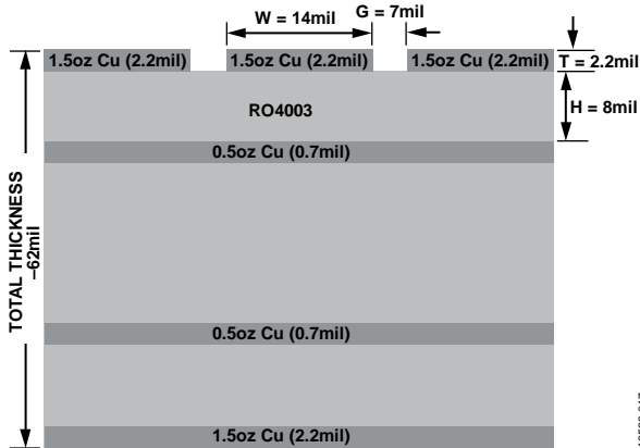
Figure 17. Evaluation Board (Cross Section View)
