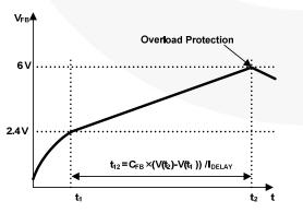
Figure 18. Overload Protection (OLP)
