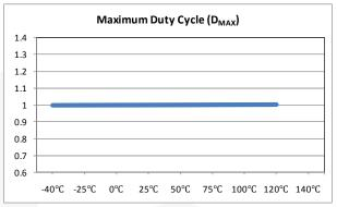
Figure 5. Maximum Duty Cycle vs. Temperature
