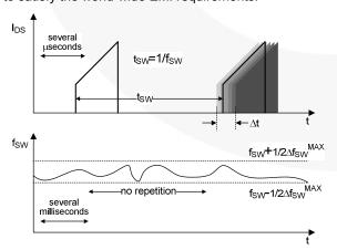
Figure 15. Frequency Fluctuation Waveform
