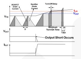
Figure 20. Output Short Waveforms (OSP)
