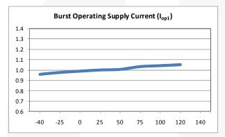
Figure 12. Burst Operating Supply Current vs. Temperature
