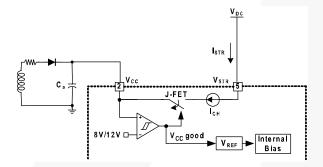
Figure 14. Startup Circuit
