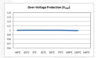
Figure 13. Over-Voltage Protection vs. Temperature
