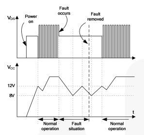
Figure 17. Auto-Restart Protection Waveforms
