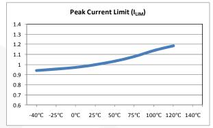
Figure 11. Peak Current Limit vs. Temperature
