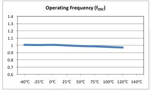
Figure 4. Operating Frequency vs. Temperature
