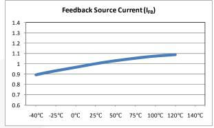
Figure 9. Feedback Source Current vs. Temperature
