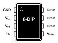
Figure 3. Pin Configuration
