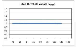
Figure 8. Stop Threshold Voltage vs. Temperature
