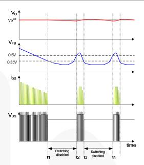
Figure 22. Burst-Mode Operation
