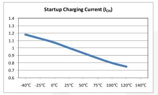
Figure 10. Startup Charging Current vs. Temperature
