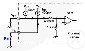
Figure 23. Peak Current Limit Adjustment
