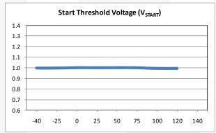
Figure 7. Start Threshold Voltage vs. Temperature
