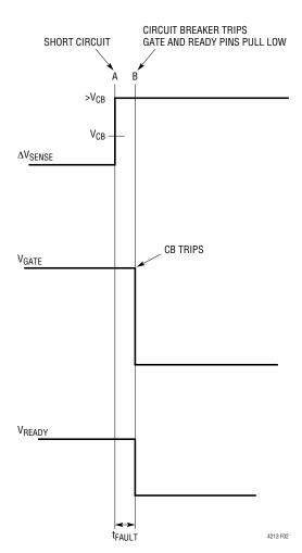
Figure 2. Short Circuit Fault Timing Diagram
