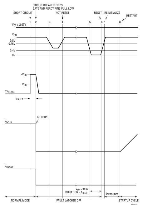
Figure 3. Resetting Fault Timing Diagram
