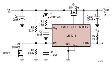
Figure 6. Single Supply Electronic Fuse
