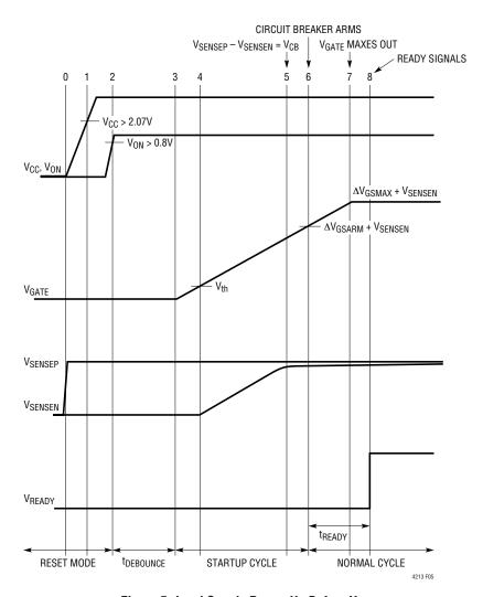
Figure 5. Load Supply Power-Up Before V<sub>CC</sub>
