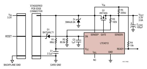
Figure 7. Single Supply Hot Board Insertion
