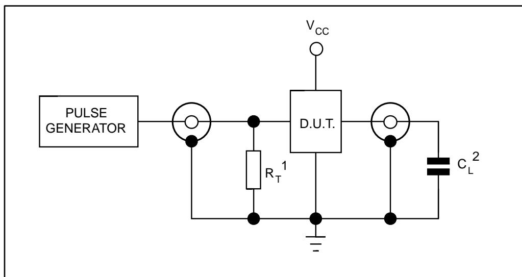
1. R<sub>T</sub> = Z<sub>OUT</sub> of pulse generator (typically 50 ohm)
