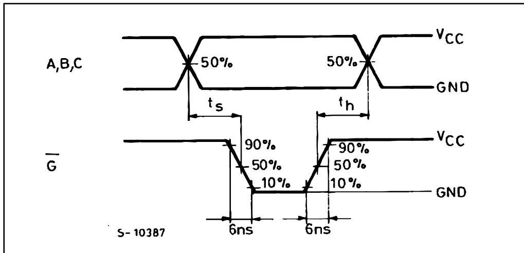
Figure 10: Waveform 6: input waveforms ( $f = 1$  MHz; 50% duty cycle)
