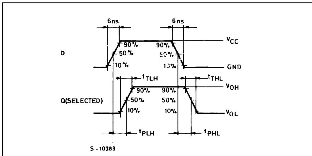
Figure 6: Waveform 2: propagation delay time ( $f = 1$  MHz; 50% duty cycle)
