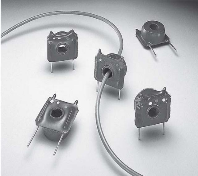
This Coilcraft current sensor is intended for measuring current from 1 to 10 amps rms. The sensor functions as the encapsulated secondary of a current transformer, while the conductor carrying the current to be measured serves as the “one turn primary.” Sensitivity may be enhanced by increasing primary turns.
