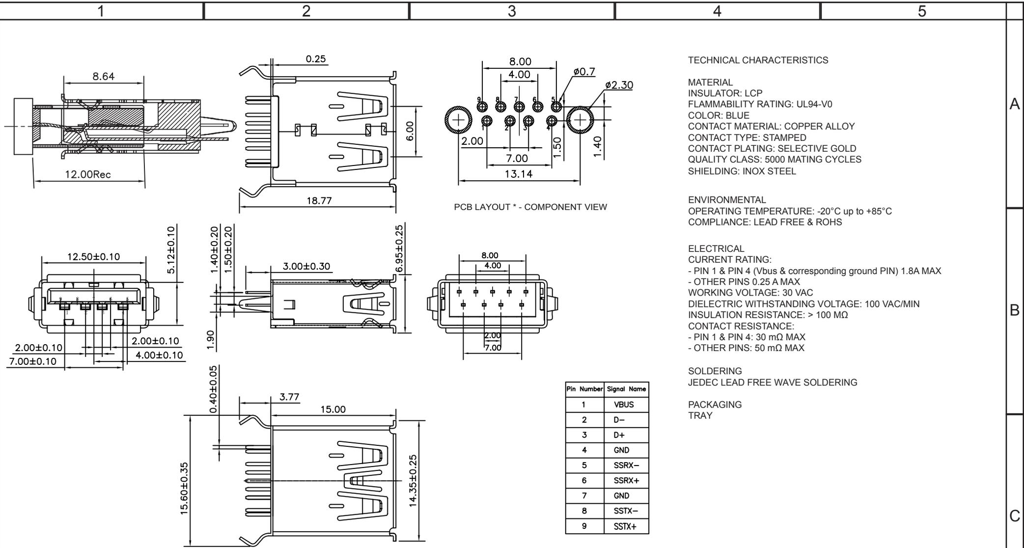
\* NOTE: THE RECOMMENDED PCB LAYOUT IS FOR AN OPTIMIZED RETENTION FORCE OF CONNECTOR ON PCB BUT IT IMPLIES INSERTION FORCE THAT A LOT OF PICK AND PLACE MACHINES ARE NOT ABLE TO HANDLE. THEREFORE IT MIGHT BE NECESSARY TO DRILL BIGGER HOLES FOR THE CLIPS. PLEASE CHECK THIS CAREFULLY.
