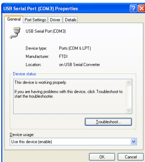
Figure 3-9 Access COM Port Properties
