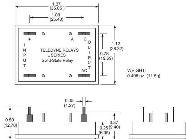
Figure 1 — Series L; dimensions in inches (mm)
