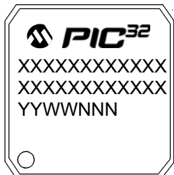
100-Lead TQFP (12x12x1 mm)
