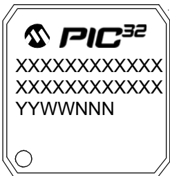
100-Lead TQFP (12x12x1 mm)
