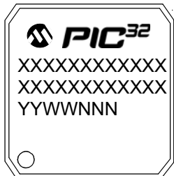
100-Lead TQFP (12x12x1 mm)
