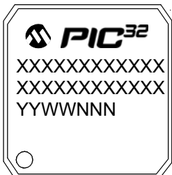
100-Lead TQFP (12x12x1 mm)
