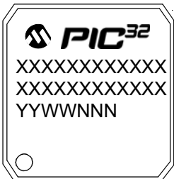
100-Lead TQFP (14x14x1 mm)
