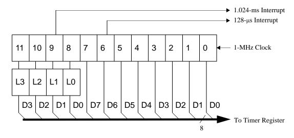
Figure 11-3. Timer Block Diagram
