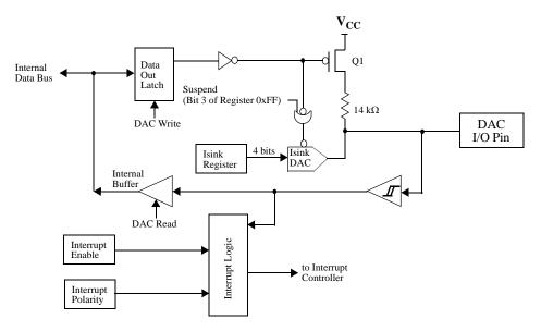
Figure 10-1. Block Diagram of a DAC Pin
