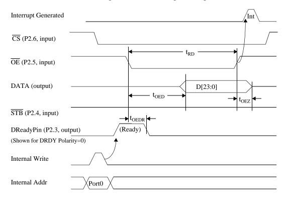
Figure 24-3. HAPI Read by External Interface from USB Microcontroller
