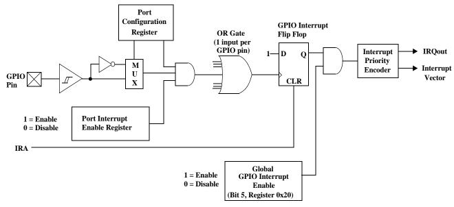
Figure 16-4. GPIO Interrupt Structure
