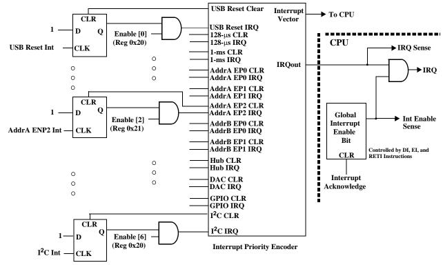
Figure 16-3. Interrupt Controller Function Diagram
