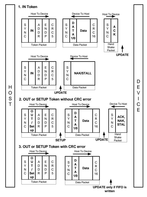
Figure 18-5. Token/Data Packet Flow Diagram
