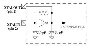
Figure 6-1. Clock Oscillator On-Chip Circuit
