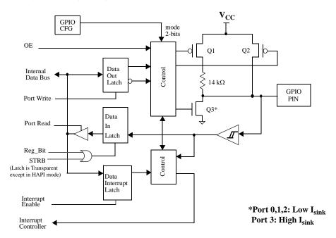
Figure 9-1. Block Diagram of a GPIO Pin
