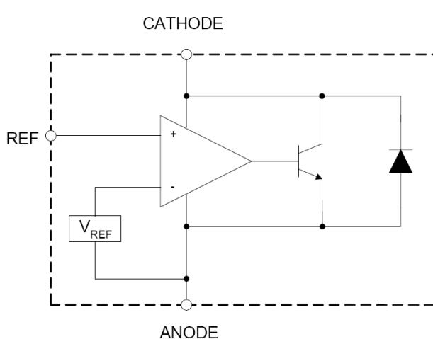
Fig. 1: XRP431L Application Diagram
