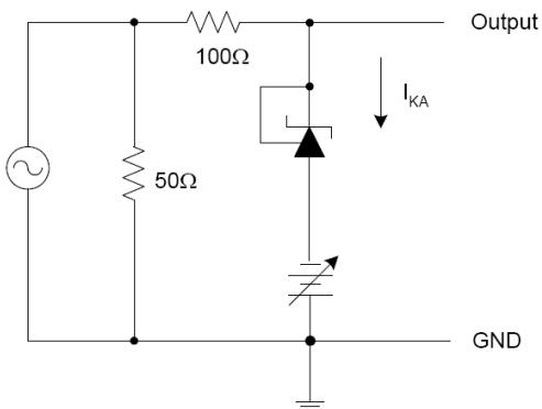
Fig. 13: Test Circuit for Dynamic Output Impedance
