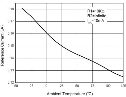
Fig. 7: Reference Input Current vs Ambient Temperature
