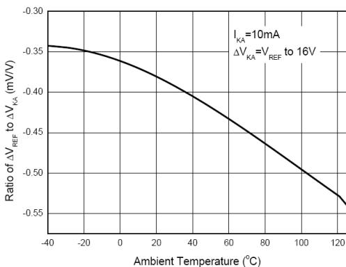
Fig. 8:  $\Delta V_{\text{REF}}$  to  $\Delta V_{\text{KA}}$  Ratio
