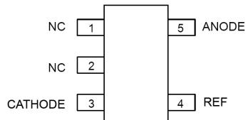
Fig. 3: XRP431L Pin Assignment
