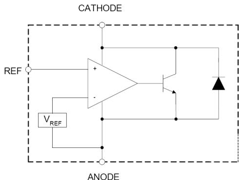
Fig. 2: XRP431L Block Diagram
