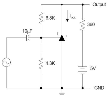
Fig. 9: Test Circuit for Gain vs Frequency Response
