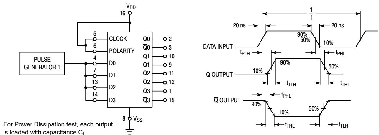
**Figure 1. AC and Power Dissipation Test Circuit and Timing Diagram
