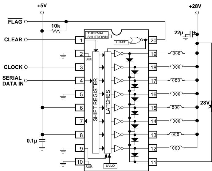
**Protected Negative/Positive PIN Diode Driver Transmit/Receive Switch**
