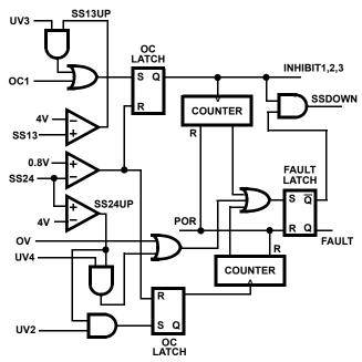
FIGURE 7. FAULT LOGIC - SIMPLIFIED SCHEMATIC
