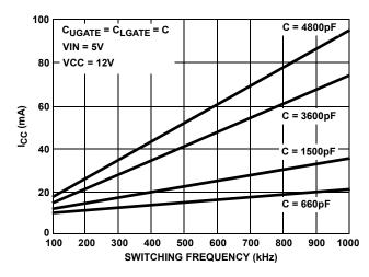
FIGURE 5. BIAS SUPPLY CURRENT vs FREQUENCY
