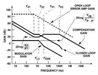
FIGURE 12. ASYMPTOTIC BODE PLOT OF CONVERTER GAIN
