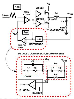
FIGURE 11. VOLTAGE-MODE BUCK CONVERTER COMPENSATION DESIGN
