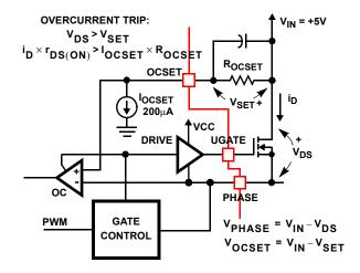
FIGURE 9. OVERCURRENT DETECTION
