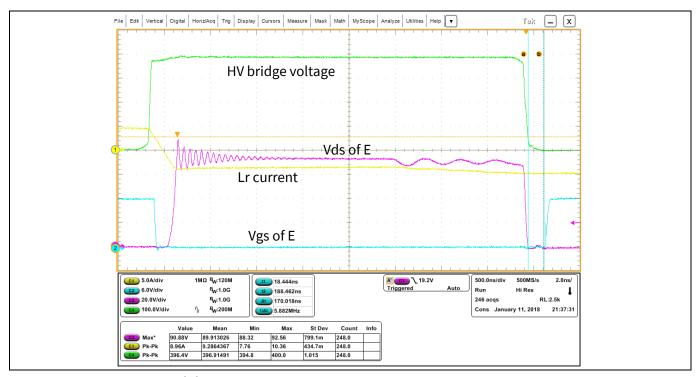
Figure 28 Standard SR driving mode
