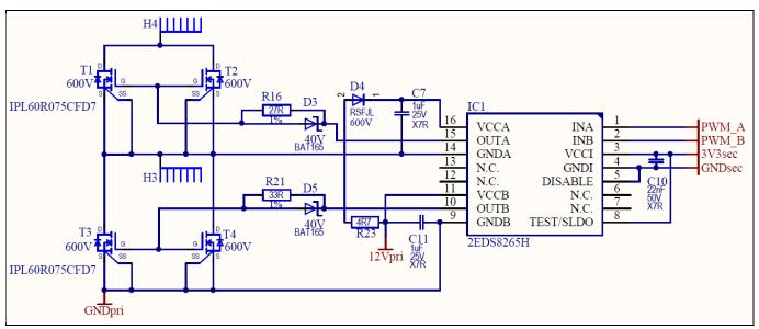
Figure 8 Driving configuration of paralleled IPL60R075CFD7 (half-bridge schematic)
