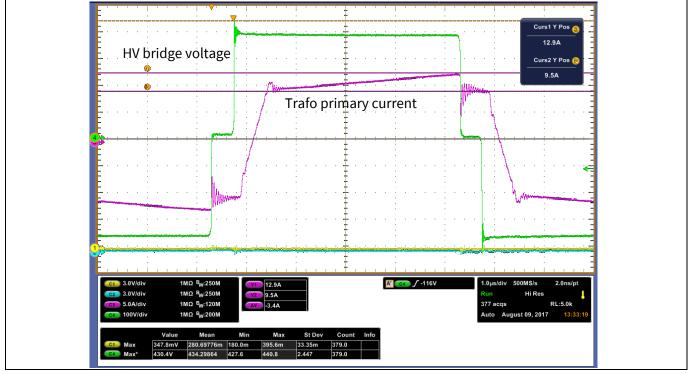
Figure 27 Full-load drain voltage of bridge overshoot
