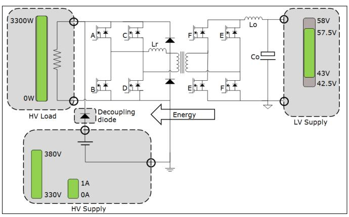
Figure 25 Boost mode recommended validation set-up
