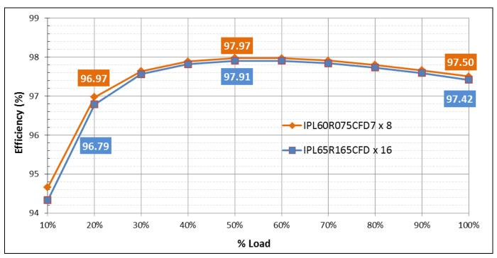
Estimated efficiency of 3300 W bi-directional PSFB in buck mode with different CoolMOS™ Figure 14 fast body diode technologies
