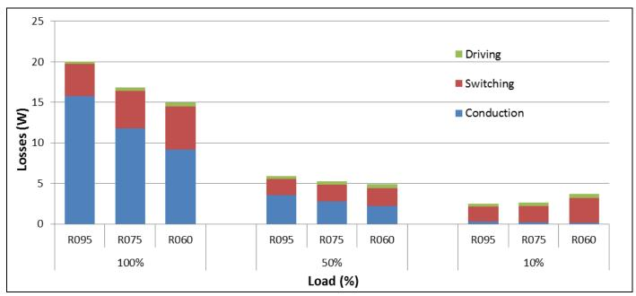
Estimated distribution of losses of 3300 W bi-directional PSFB in buck mode with different Figure 12 CoolMOS™ CFD7 R<sub>DS(on)</sub> in ThinPAK
