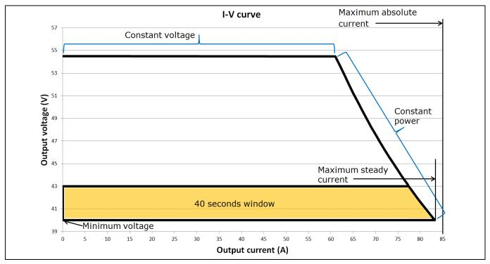
Figure 32 Constant voltage, constant power curves
