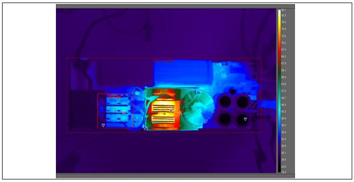
Figure 33 Thermal capture at 61 A load with open case and external fan – front view
