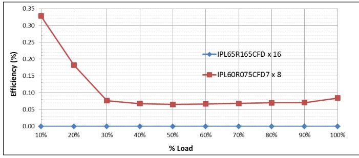
Different estimated efficiencies of 3300 W bi-directional PSFB in buck mode with different Figure 13 CoolMOS™ fast body diode technologies
