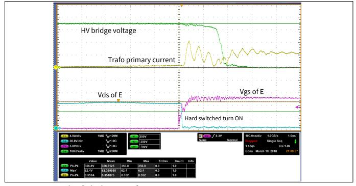
Figure 37 Hard-switched turn-on of LV MOSFETs
