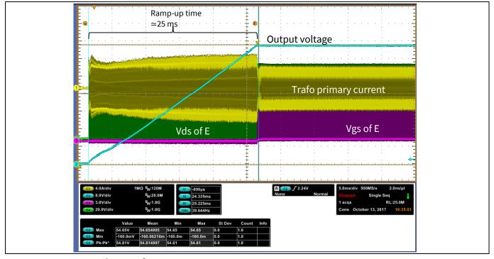
Figure 30 Output voltage soft-start-up
