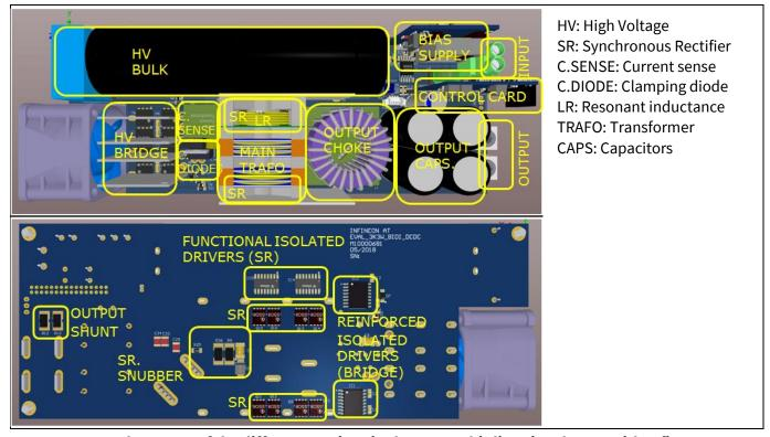
Placement of the different sections in the 3300 W bi-directional PSFB with Infineon Figure 5 CoolMOS™ CFD7 and OptiMOS™ 5
