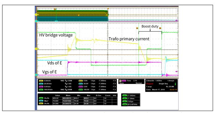
Figure 35 Boost mode duty cycle. Transformer primary current (yellow), LV MOSFET drain voltage (blue), LV MOSFET gate voltage (pink), bridge voltage (green). Note: capture taken at scaleddown voltages.
