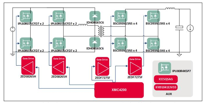
3300 W bi-directional PSFB (EVAL 3K3W BIDI PSFB) - simplified diagram showing the Figure 3 Infineon semiconductors used
