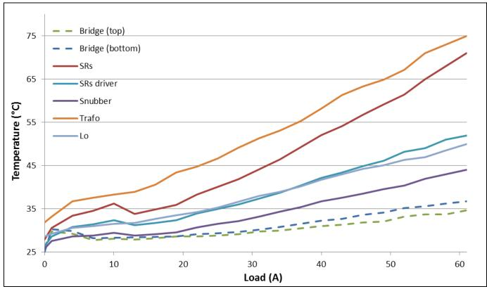
Measured temperatures on PSFB 3300 W converter at 25°C room temperature and with Figure 21 open case
