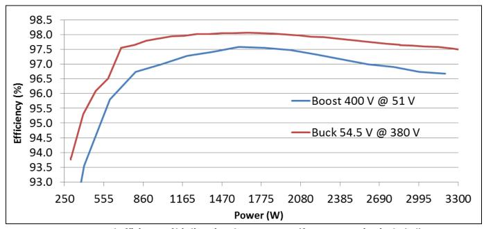
Figure 2 Measured efficiency of bi-directional 3300 W PSFB (fan consumption included)
