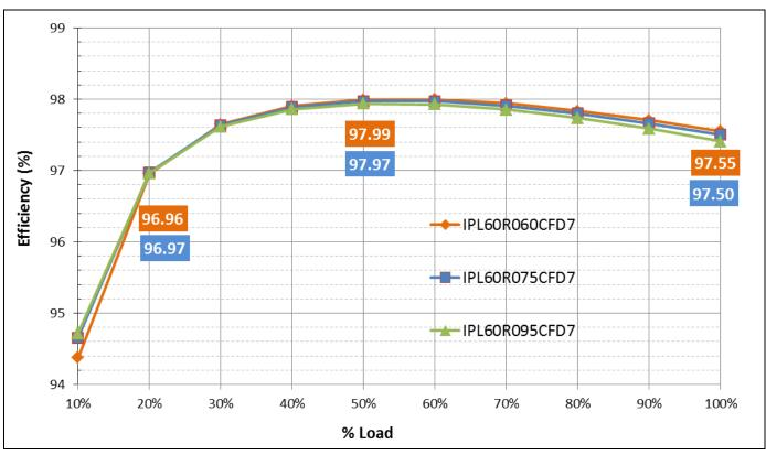
Estimated efficiency of 3300 W bi-directional PSFB in buck mode with different CoolMOS™ Figure 10 CFD7 R<sub>DS(on)</sub> in ThinPAK
