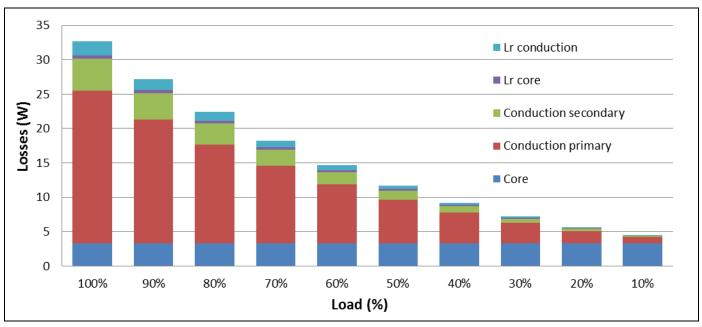
Figure 16 Estimated distribution of losses of stacked magnetic structure: transformer and resonant inductance
