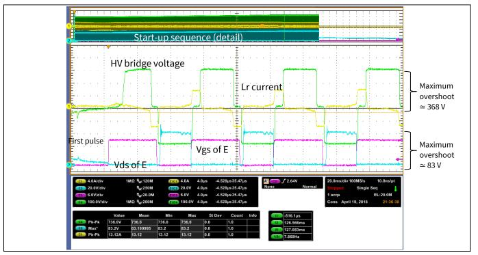
Soft-start sequence, first pulses ensuring near ZVS for bridge transitions. Note: scaled Figure 39 voltages test capture.
