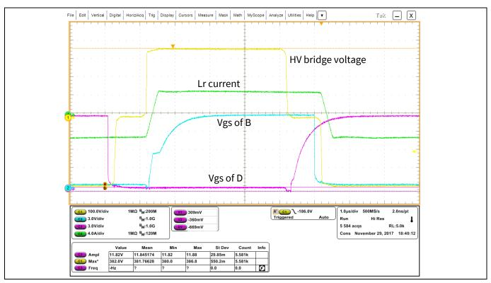
Figure 26 ZVS turn-on of lagging leg (D switch) and partially hard-switched turn-on of leading leg (B switch)
