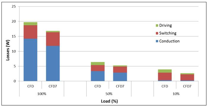
Estimated distribution of losses of 3300 W bi-directional PSFB in buck mode with different Figure 15 CoolMOS™ fast body diode technologies
