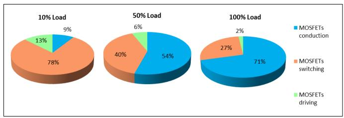
Figure 7 IPL60R075CFD7 loss distribution (percentage of MOSFET contribution) along load in the 3300 W bi-directional PSFB in buck mode
