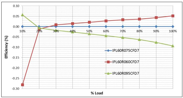
Figure 11 Different estimated efficiencies of 3300 W bi-directional PSFB in buck mode with different CoolMOS™ CFD7 R<sub>DS(on)</sub> in ThinPAK
