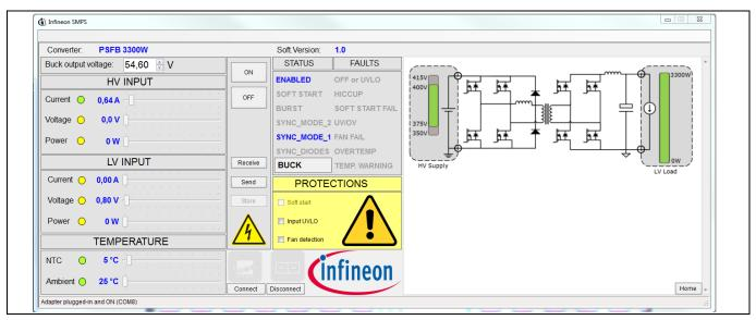
Figure 44 3300 W bi-directional PSFB simplified user interface
