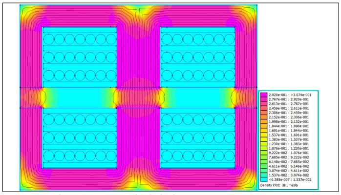
Figure 18 Main transformer flux density distribution – FEMM
