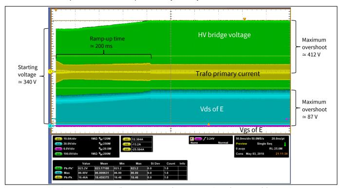
Soft-start sequence, first pulses ensuring near ZVS for bridge transitions Figure 38
