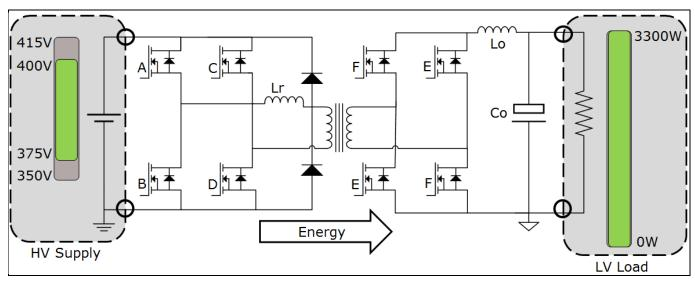
Figure 24 Buck mode recommended validation set-up
