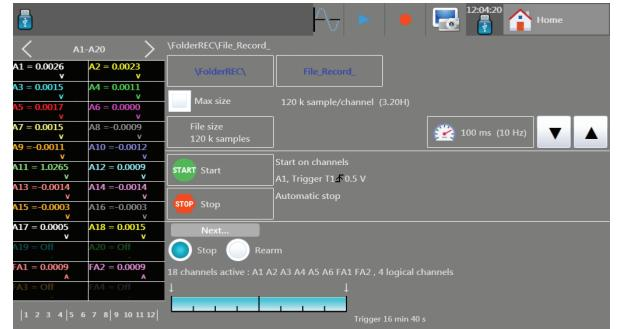
Comprehensive triggering capabilities: Configure triggers on analog and logic channels. Select from multiple combinations of thresholds, channels and conditions.
