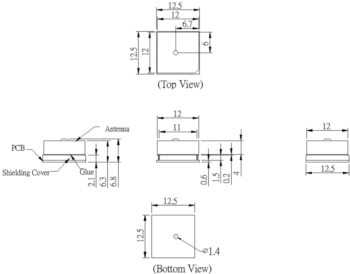
Fig. 2.1 Mechanical Dimension
