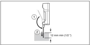
Figure 3. Extended Contact Probe
