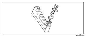
Figure 14. Probe Replacement
