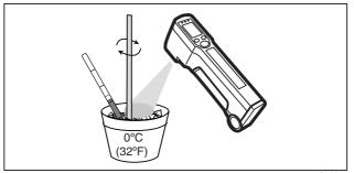
Figure 8. Cold Temperature Verification Check
