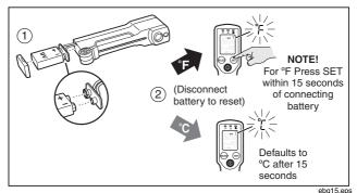
Figure 12. Setting/Changing °C and °F Temperature Scales
