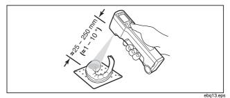
Figure 10. Noncontact Thermometer Working Range
