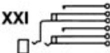
Double open circuit. Isolated switching—separate "make" circuits on both tip and ring. (J2-2A).
